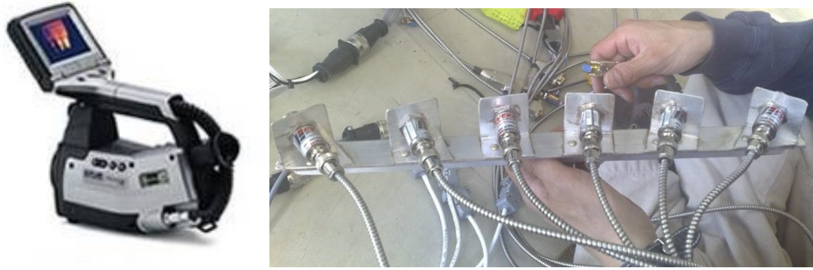
Figure 2-4: Thermal imager (left) without the 80° FOV lens attached and thermal infrared radiometers (right).
