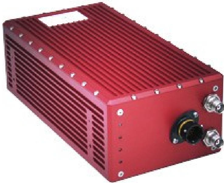
Figure 2-2: The RT3003 OXTS Inertial + GPS system. Refer to www.oxts.com for more information.
