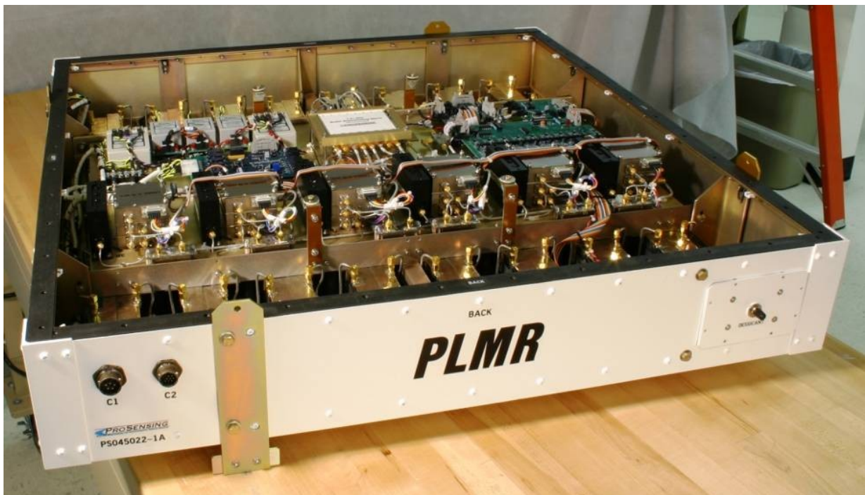
Figure 2-3: View of PLMR with the cover off.
