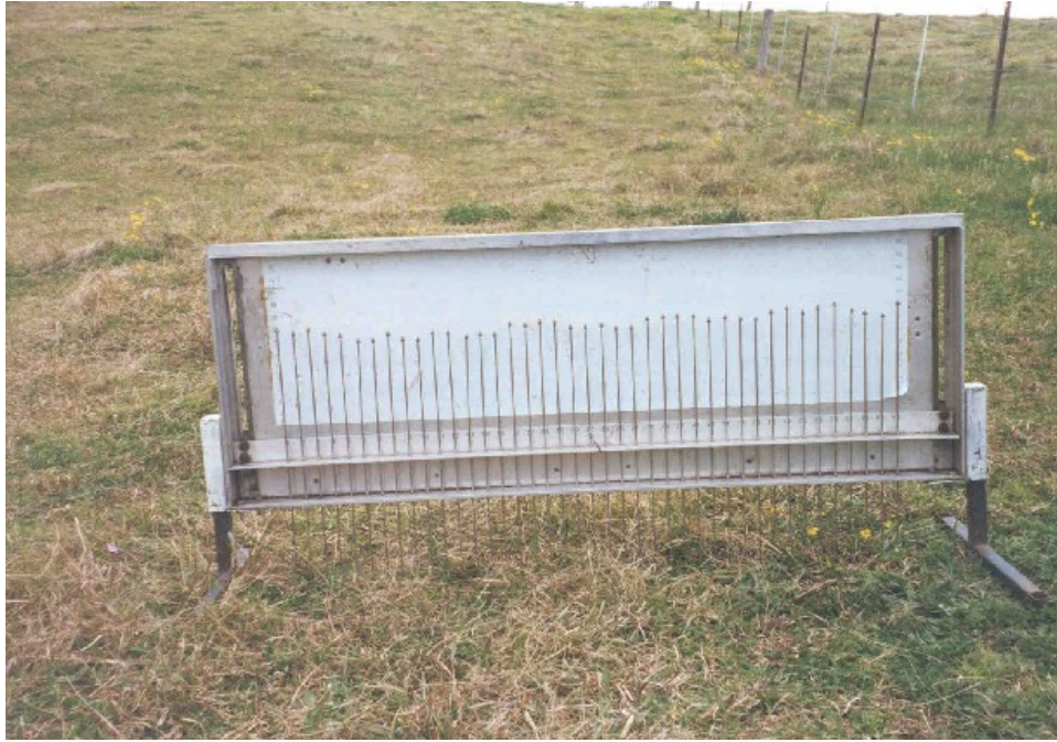
Figure 7-4: Pin profiler for surface roughness measurements.
