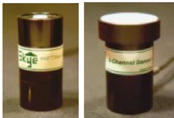
Figure 2-5: Multi-spectral sensors; downward looking sensor without the field of view collar attached (left) and upward looking sensor with cosine diffuser fitted (right).
